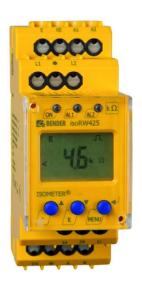
Insulation monitoring device for unearthed IT AC-, AC/DC and DC systems (IT systems) for railway applications up to 3(N)AC, AC/DC 440 V Software version: D0418 V2.xx
