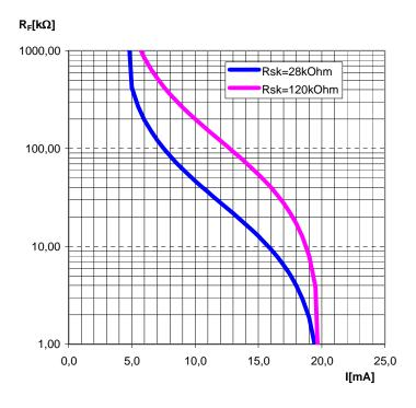
$$R_F = \frac{16 \text{ mA x R}_{Sk}}{1 - 4 \text{ mA}} - R_{Sk}$$
