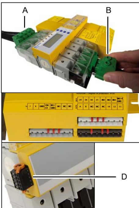
Connect the terminals according to the wiring diagram to the plug connectors (A, B) and the connector plugs (C, D).
