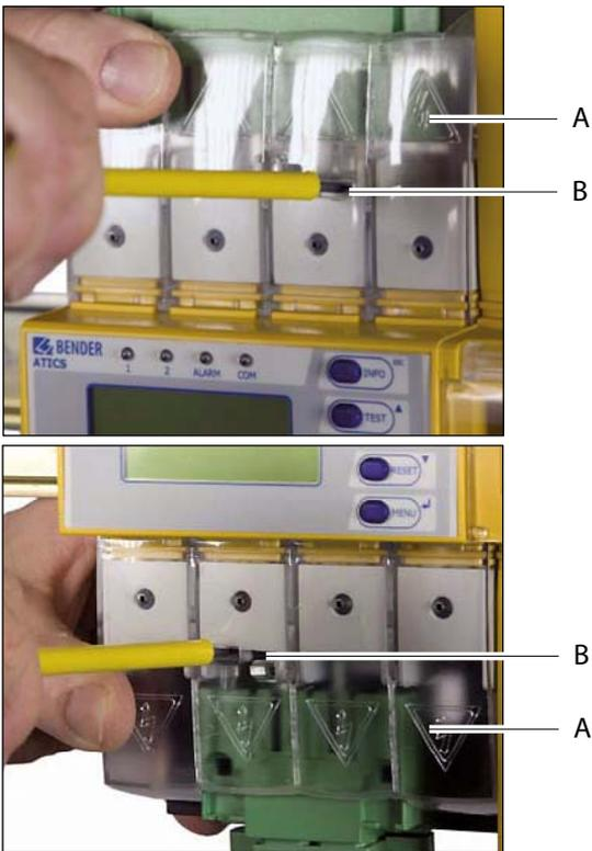
1. Push back the locking hook (B) in the middle of the top and bottom terminal cover (A) by using a screwdriver.
