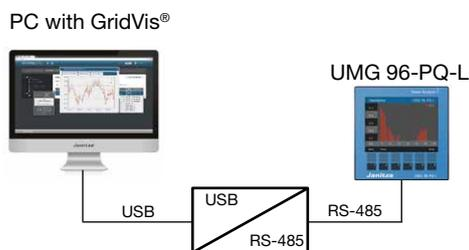
1. Use of the UMG 96-PQ-L (server device) via a UMG with gateway functionality (e.g. UMG 512 client device):
