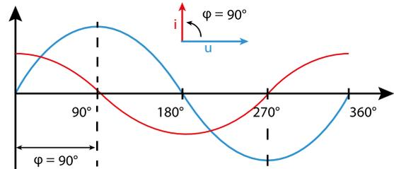
With a combination of the states, the phase angle “current to voltage” can assume values between  $-90^\circ$  and  $+90^\circ$ .
