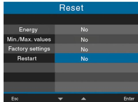
Fig. Reset window, restart device
