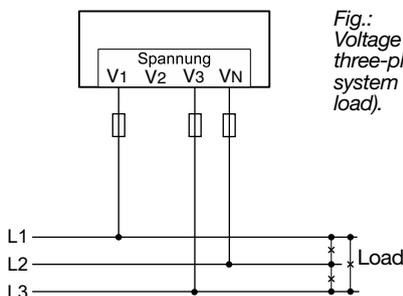
Fig.: Voltage measurement in a three-phase 3-conductor system (asymmetrical load).
