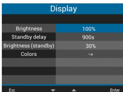
Settings for brightness, standby time after, brightness (standby) and the display colors for voltage and current (L1, L2, L3).
