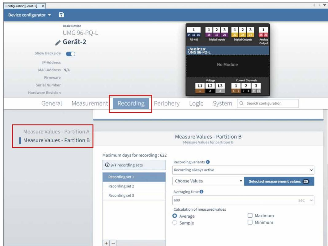
Fig. Recording configuration of memory partition B in the GridVis<sup>®</sup> software
