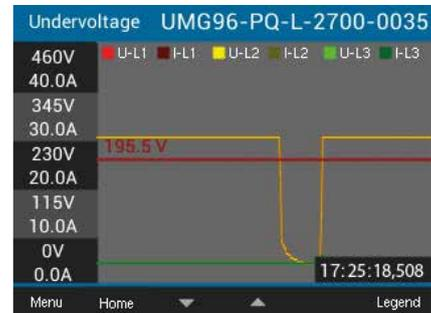
Display – sequence of an undervoltage in the three-phase 4-wire system
