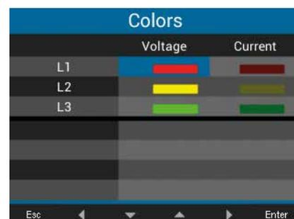
Settings for the display colors of voltage and current (L1, L2, L3).
