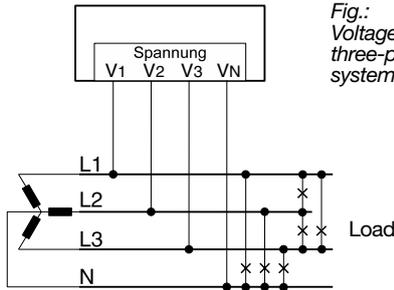
Fig.: Voltage measurement in three-phase 4-conductor system
