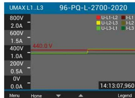
Display – sequence of an overvoltage in the three-phase 3-wire system
