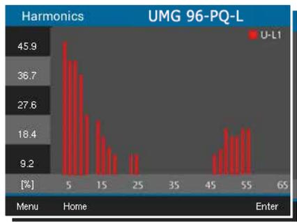
Display of the harmonics up to the 65th harmonic (voltage L1, L2, L3)
