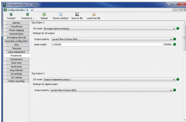
Fig. Configuration of the digital outputs via the GridVis<sup>®</sup> software
