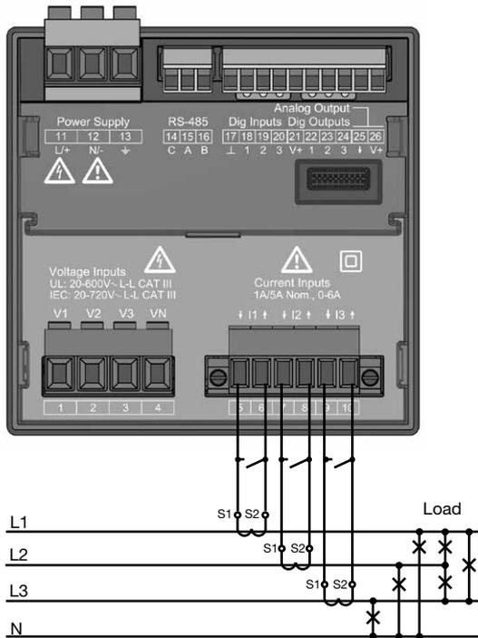
Fig. Connection example, "Current measurement via current transformer".
