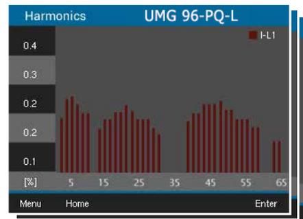
Display of the harmonics up to the 65th harmonic (current L1, L2, L3)
