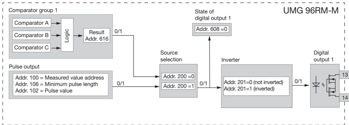
Fig.: Overall block diagram for digital output 1
