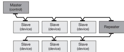
*Illustration of bus type: Line structure*
