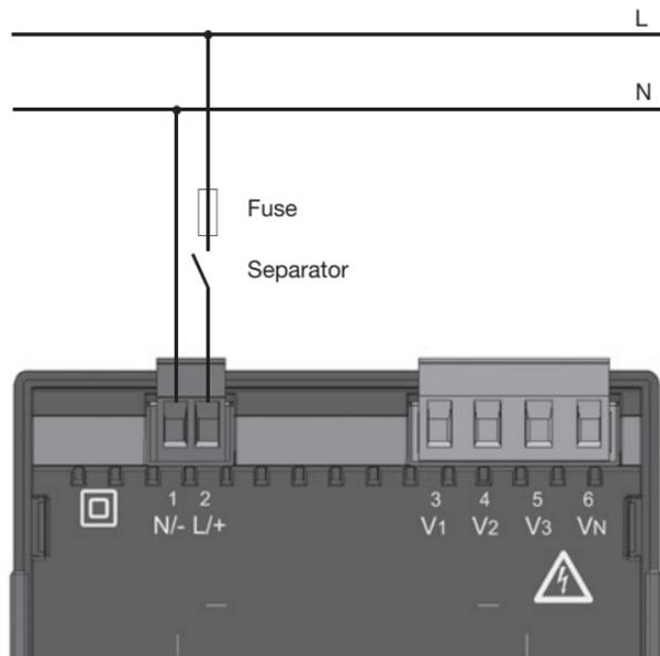
*Fig. Connection example of the supply voltage to the UMG 96RM-M*
