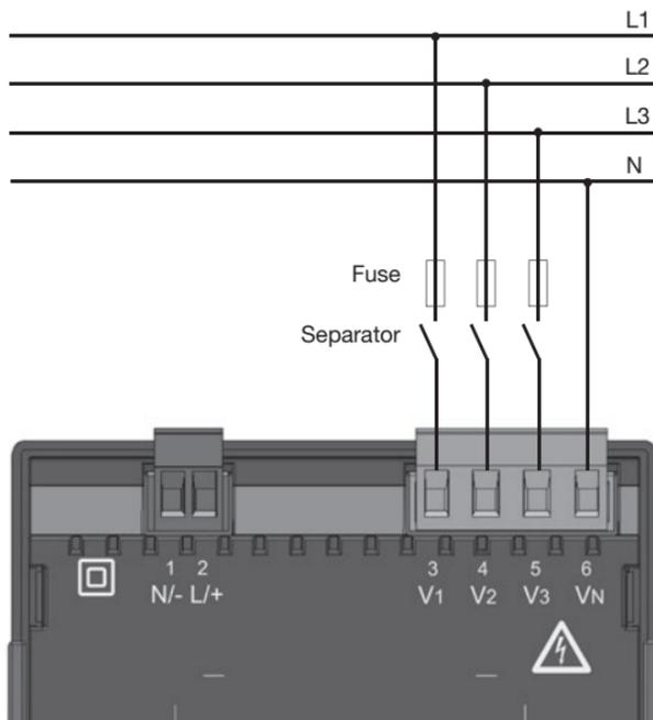
Fig. Connection example for the voltage measurement
