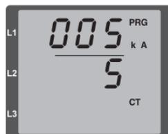
*Fig. Current transformer programming mode*
