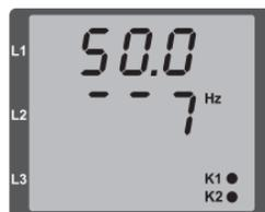
*Fig. Display of the mains frequency (50.0) and the rotation field direction*
