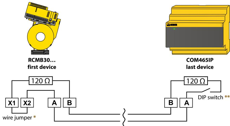
\* The internal 120 Ω terminating resistor can be connected by using the wire jumper.
