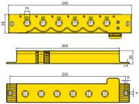
Fig. 4.1: Dimension diagram RCMS150
