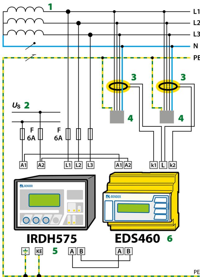
EDS system with IRDH575, EDS460 and measuring current transformers W... in a 3AC system
