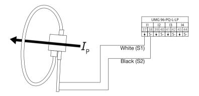
The connecting cable is shielded. The shield is already connected to the blue wire and insulated with shrink tubing. This results in the colors black and white. The ends are fitted with wire end ferrules.
