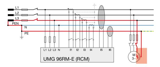
Fig.: UMG 96RM-E with residual current monitoring via measuring inputs 15 / 16
