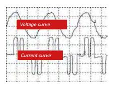
Fig. 10: Grid distortions through frequency converters
