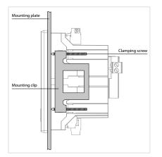
Fig.: The mounting into a switchboard is done via the lateral fastening clips (UMG 96RM-P / UMG 96RM-CBM)
