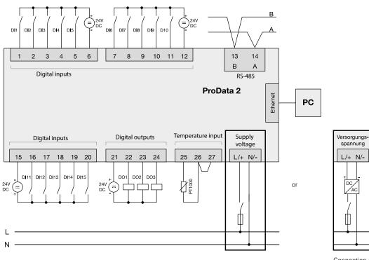
Connection example via external power supply
