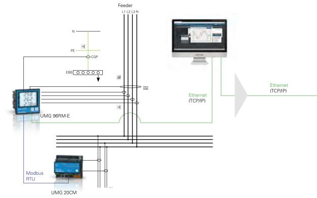
Fig.: The 20 channels of the UMG 20CM can be optionally used for residual or operating current monitoring using the corresponding current transformers. Residual current monitoring detects the residual currents flowing to ground or via other paths.
