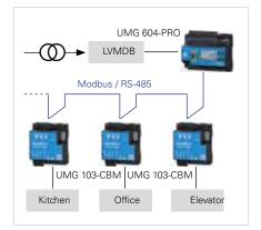
Fig.: Topology example for UMG 604-PRO (master) – UMG 103-CBM (slave)
