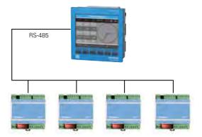
Fig.: The I/O fieldbus modules are connected via the RS-485 interface of the UMG measurement device
