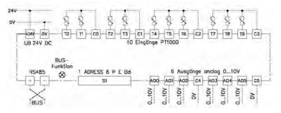
Fig.: Connection example of FBM10 PT1000/PT100; thermistor input, 2-wire
