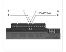
Fig.: RS-485 interface, 2-pole plug contact
