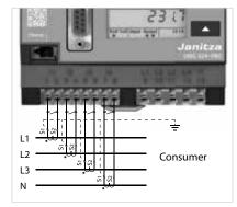
Fig.: Current measurement via current transformers
