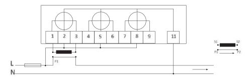
Fig.: 2-wire connection / 1 measuring unit
