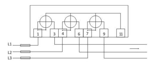
Fig.: 3-wire connection / 2 measuring units
