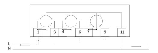
Fig.: 2-wire connection / 1 measuring unit
