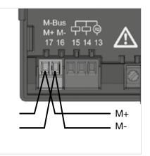
Fig.: M-Bus interface with 2-pole plug contact
