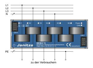
Fig.: Operating current measurement, e.g. 6 x 1-phase
