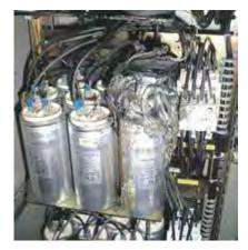
Fig. 6: Destroyed PP reactive power compensation capacitor: A creeping highimpedance ground fault has led to the complete melting of the capacitor and a localized fire.
