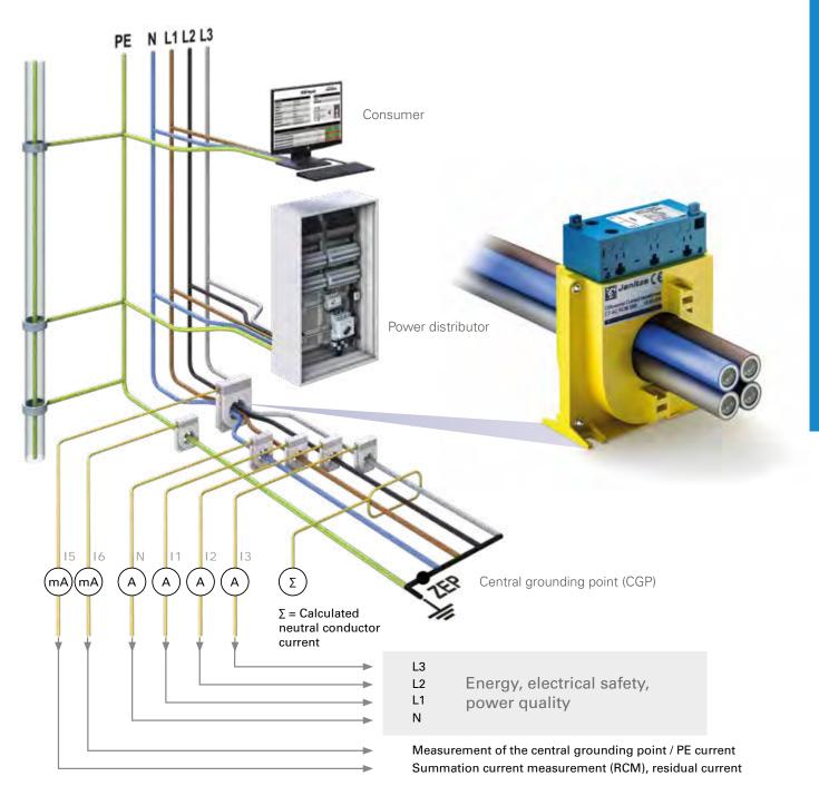
Residual and operating current monitoring: Can be implemented with the UMG 512-PRO / UMG 509-PRO / UMG 96RM-E and UMG 96-PA network analyzers (with RCM module). The RCM device used should be easy to handle, automatically point out problems and at the same time provide valuable assistance to the service technician.
