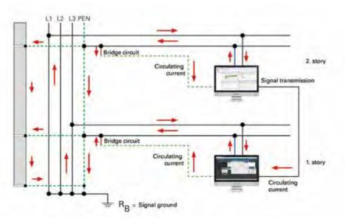
Fig. 12: Operating currents on grounding systems
