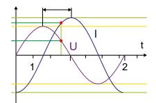
Fig.: Phase shift between current and voltage (  $\Delta \phi )$
