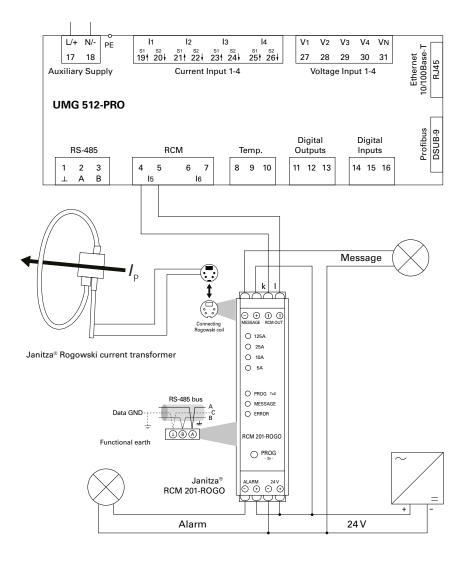
Fig.: Connection example to a UMG 512-PRO
