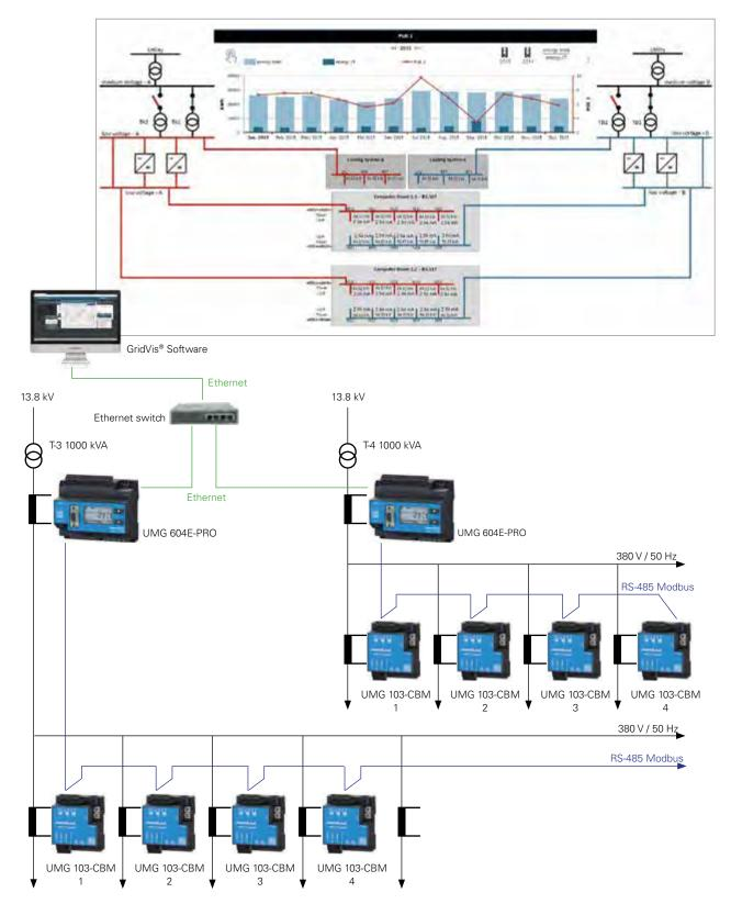
Fig.: Illustration of typical application with 2 feeders, UMG 604-PRO as master meters in the main feeder and UMG 103-CBM for measuring the low voltage outgoing feeders.
