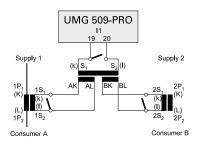
Fig.: UMG 509-PRO current measurement summation transformer
