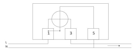
Fig.: 2-wire connection / 1 measuring unit
