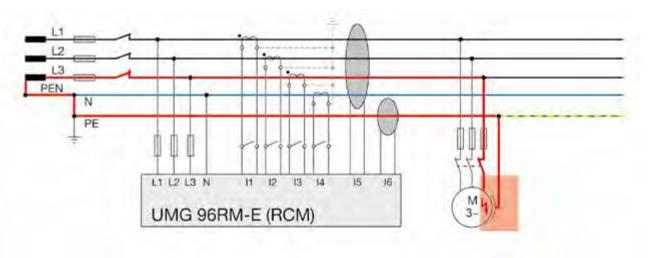
Fig. 3: Faulty motor insulation leads to a ground fault and fault current to the PE conductor
