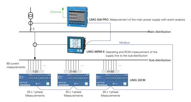
Fig.: Extremely compact solution for complete monitoring over three levels with state-of-the-art master-slave communication architecture
