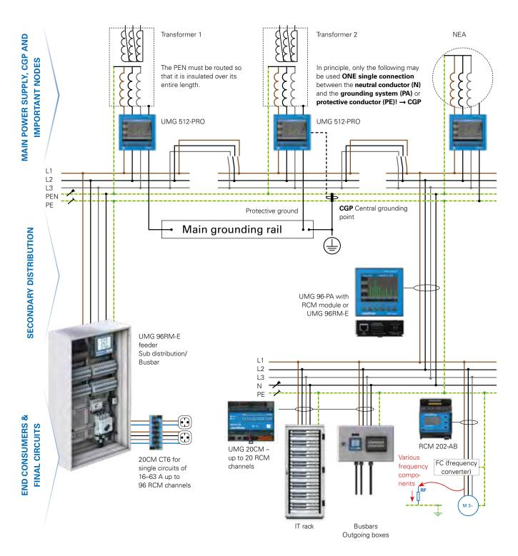
Fig.: Holistic energy & residual current monitoring
