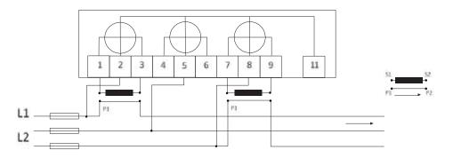
Fig.: 3-wire connection / 2 measuring units
