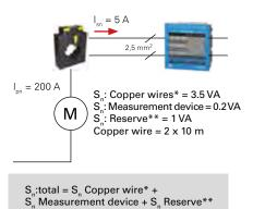
Example:  $S_n \text{ total} = 3.50 \text{ VA} + 0.2 \text{ VA} + 1 \text{ VA}$  $S_n \text{ total} = 4.70 \text{ VA}$  (corresponds to the standardized value of 5 VA)
