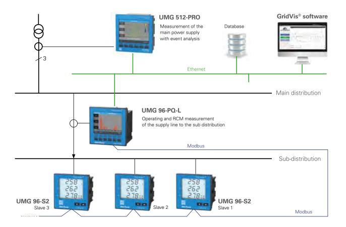
Fig.: Master slave principle
