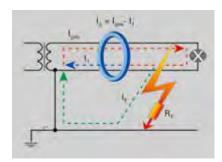
Fig. 2: Principle of residual current measurement
