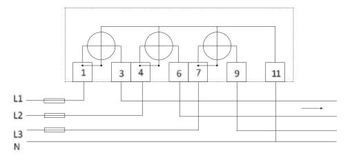
Fig.: 4-wire connection / 3 measuring units
