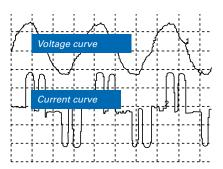
Fig.: Grid distortions due to frequency converters
