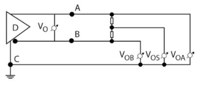
VO = Differential voltage A - B VOB = Voltage between B and C VOA = Voltage between A and C VOS = Driver offset voltage
