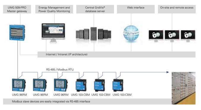
Fig.: Master-slave communication architecture
