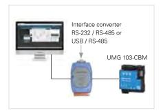
Fig.: Connection of a UMG 103-CBM to a PC via an interface converter
