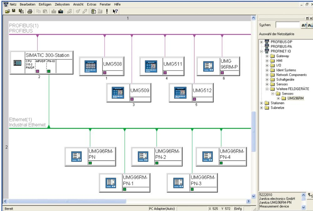
Complete integration of the Janitza measurement devices in the Step 7® software environment
