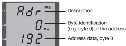
Fig. TCP/IP address, byte 1
