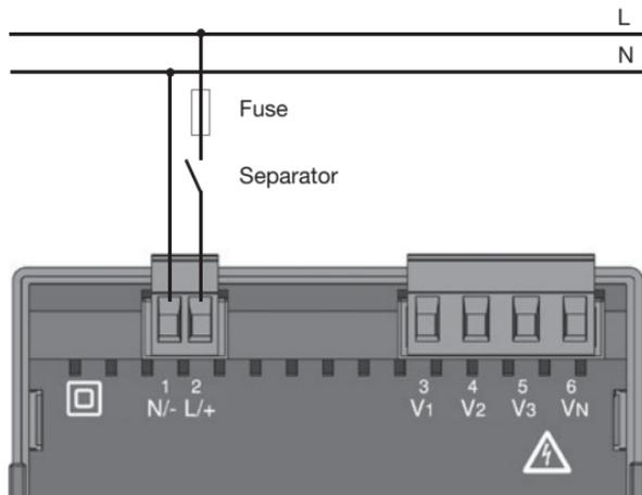
*Fig. Connection example of the supply voltage to the UMG 96RM-EL*
