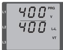
*Fig. Programming mode Voltage transformer*
