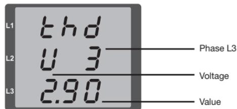
Fig. Display of the total harmonic distortion of the voltage from the L3 phase (example).
