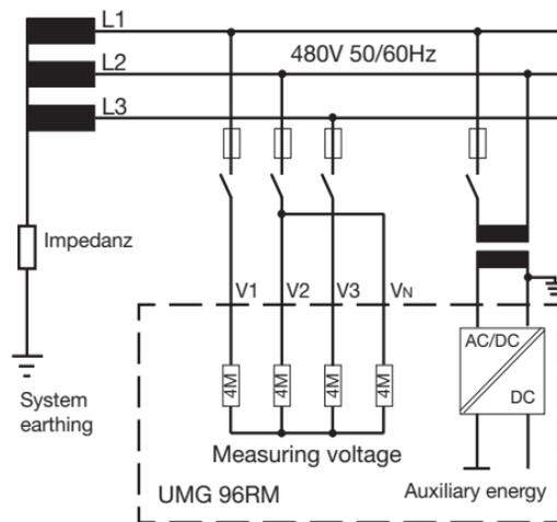
Fig. Principle circuit diagram - Measurement in three-phase 3-wire systems.
