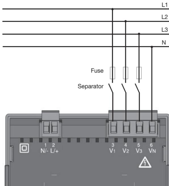
Fig. Connection example for the voltage measurement
