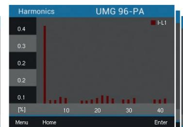
Display of harmonics up to the 40th harmonic. (Current L1, L2, L3)
