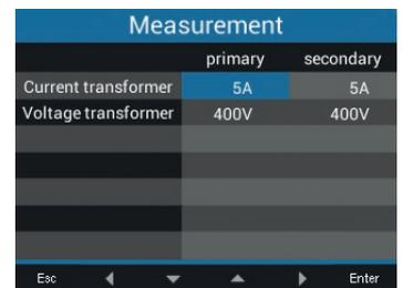
Current and voltage transformers (primary and secondary) setting.
