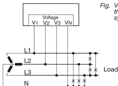
Fig. Voltage measurement in the three-phase 4-conductor system
