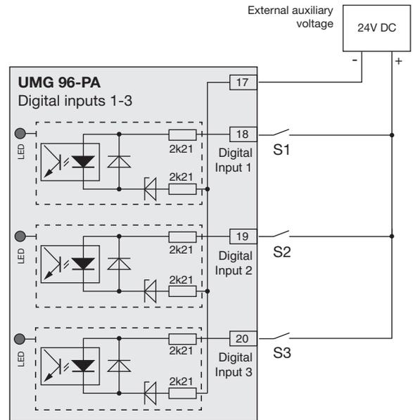
Fig. Example for connecting the external switching contacts S1-S3 to the digital inputs 1, 2 and 3.
