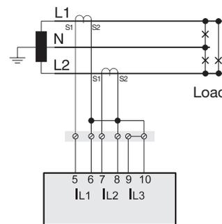
Fig. Current measurement in the single-phase 3-conductor system
