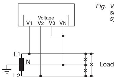
Fig. Voltage measurement in the single-phase 3-conductor system
