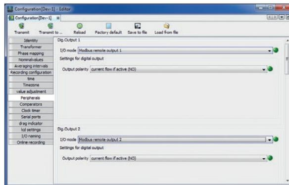
Fig. Configuration of the digital outputs as a "Modbus remote" in GridVis® software
