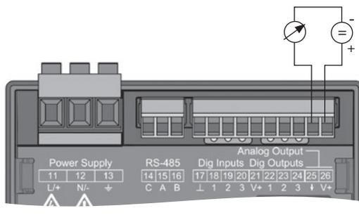
Fig. Analog output connection
