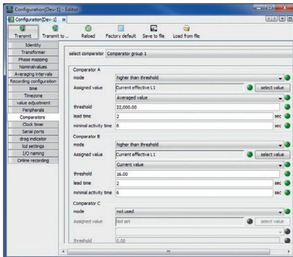
Fig. Configuration of the comparator in the GridVis® software
