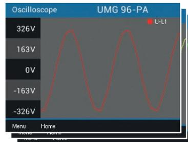
Display of the voltage L1, L2 or L3 oscillogram
