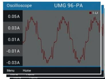
Display of current L1, L2, L3 oscillogram
