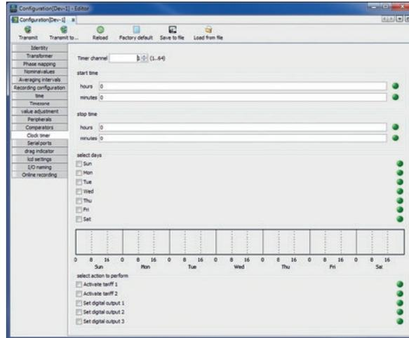
Fig. Configuration of the weekly timer (GridVis® software)
