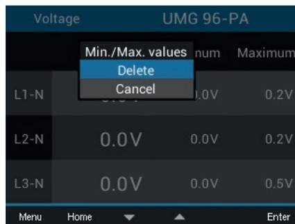
Fig. Voltage L-N measured value indication with delete/cancel *Min./Max. values* menu
