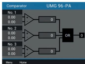
Display of threshold value, actual value, comparator runtime, logic and status
