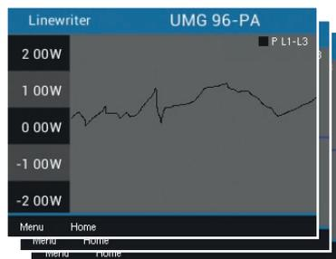
Display of the active, reactive or apparent power curve (sum L1..L3)
