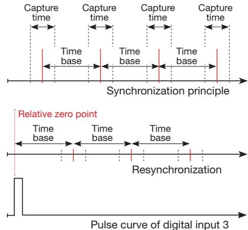
Fig. Synchronization principle with "a pulse outside the capture time"
