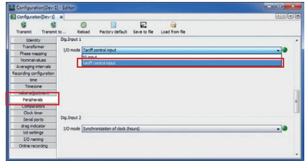
Fig. Configuration of digital input 1 as the tariff changeover input in the GridVis® software
