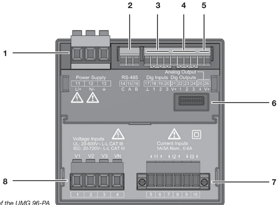
Fig. Rear view of the UMG 96-PA
