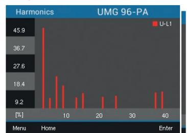
Display of harmonics up to the 40th harmonic. (Voltage L1, L2, L3)
