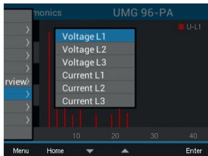
Fig. Selection list with voltages and currents for displaying the harmonics.
