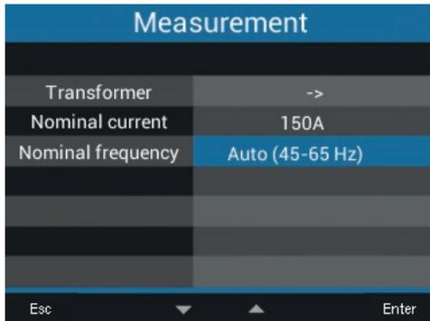
Fig. Configuration window with the rated frequency entry activated.
