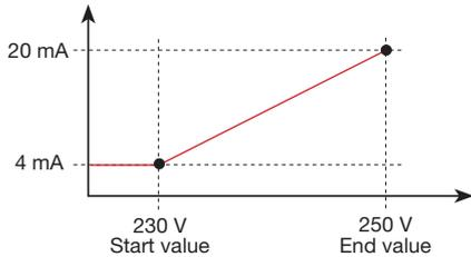
Fig. Analog output principle with voltage monitoring
