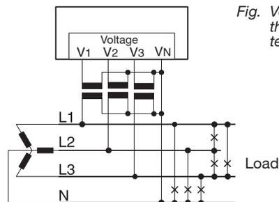
Fig. Voltage measurement in the three-phase 4-conductor system via voltage transformers
