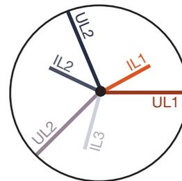
Current and voltage are shifted against each other. The current rushes ahead of the voltage, i.e. the network is capacitively loaded.
