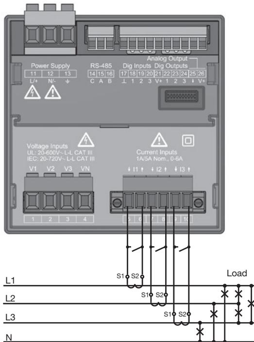
Fig. "Current measurement via current transformer" connection example
