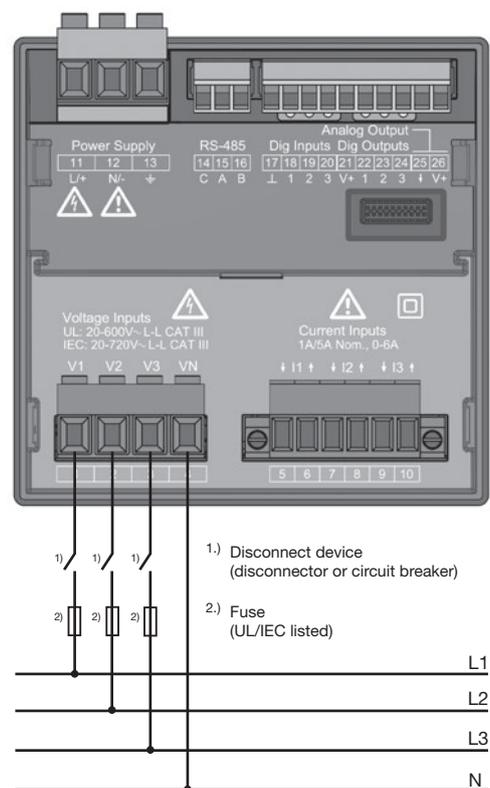
Fig. Connection example for the voltage measurement.
