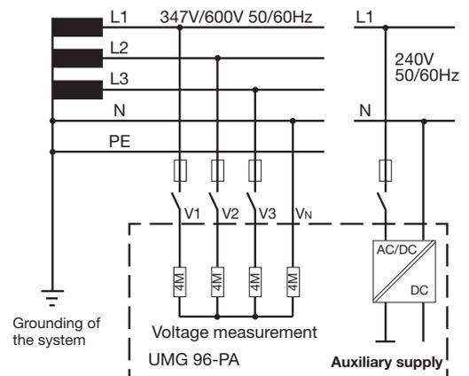
Fig. Schematic diagram - measurement in three-phase 4-conductor systems.
