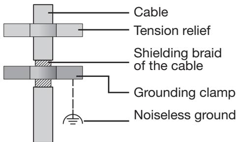
Fig. Shielding design at cabinet entrance.
