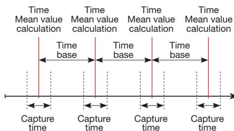
Fig. Synchronization principle
