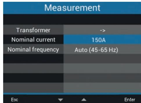
Fig. Measurement window with the rated current entry activated.
