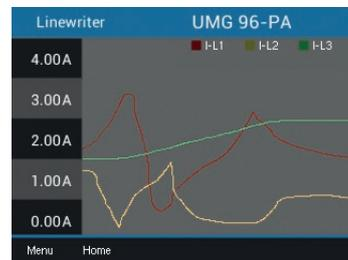
Display of current curve of L1, L2, L3
