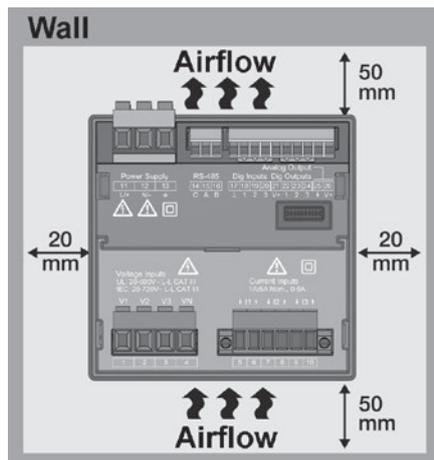
Fig. Rear view of the UMG 96-PA mounting position
