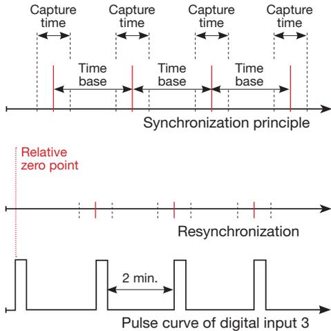
Fig. Synchronization principle with “periodic pulses” on digital input 3
