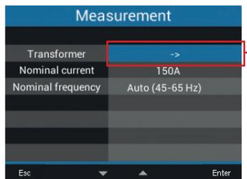
Measuring transducer, rated current and rated frequency settings.
