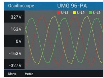
Display of the voltage L1, L2 and L3 oscillogram
