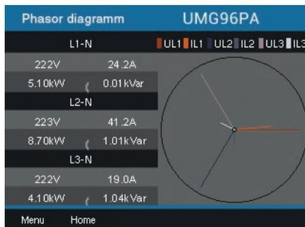
Fig. The phasor diagram shows voltages with long pointers and currents with short pointers.
