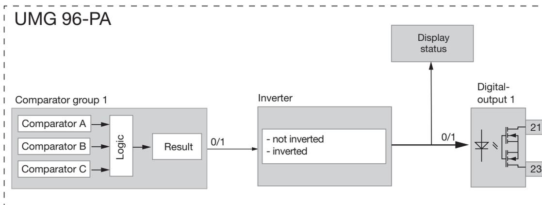
Fig. Block diagram "Use of digital output 2 for threshold value monitoring".
