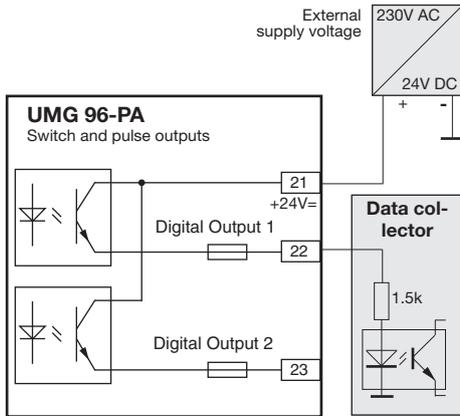
Fig. Connection example for switching as a pulse output.
