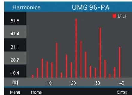
Fig. Harmonics measured value indication (e.g. voltage L1)
