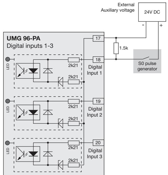
Fig. Example for connecting an S0 pulse generator the digital input 1.
