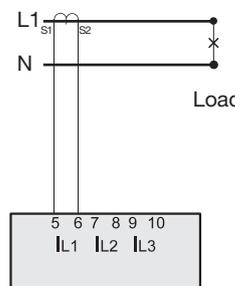
Fig. Current measurement in the single-phase 2-conductor system
