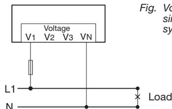
Fig. Voltage measurement in the single-phase 2-conductor system
