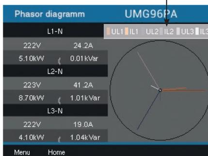
Fig. Phasor diagram window showing the phase sequence according to the rotation field direction.
