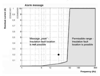
A measuring channel where insulation fault location is not possible is marked with "peak" in the "Alarm/meas. values" menu.
