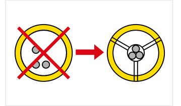
The cables must be aligned with the centre of the measuring current transformer.
