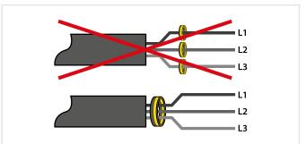
All current-carrying cables must be routed through the measuring current transformer.
