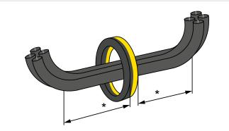
\* Distance to 90° angle: 2x external diameter of the current transformer
