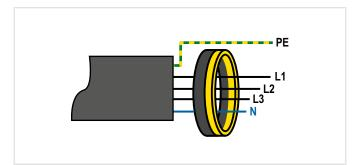
Never route an existing protective conductor through the measuring current transformer.
