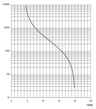
$$R_F = \frac{16 \text{ mA x } 2800 \text{ k}\Omega}{\text{I - 4 mA}} \text{ - 2800 k}\Omega$$
