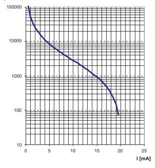
$$R_F = \frac{20 \text{ mA x } 2800 \text{ k}\Omega}{\text{I}} - 2800 \text{ k}\Omega$$
