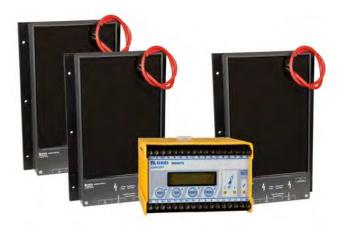
Insulation monitoring device for medium voltage IT systems with galvanically connected rectifiers and converters up to AC/DC 15.5 kV in combination with the coupling devices AGH675S-7 and AGH675S-7MV15
