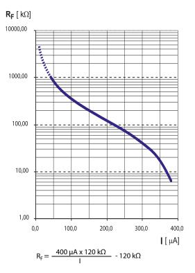
$R_{\rm F}$  =Insulation fault in k $\Omega$ *I* =Current output in mA
