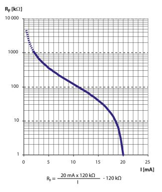
$R_{\rm F}$  =Insulation fault in k $\Omega$ I =Current output in mA
