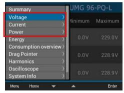
Fig. Voltage, current and power menus
