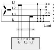
Fig.: Current measurement via 2 current transformers (Aron circuit) in a three-phase 4-conductor system
