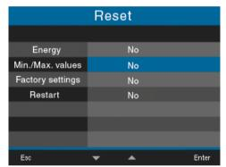
Fig. Reset window, delete min/max values
