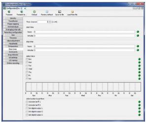
Fig. Configuration of the weekly timer (GridVis ® software)
