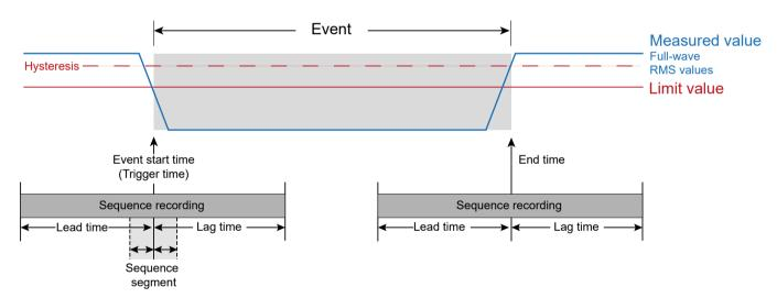
Example 2 of an event (> 20 s) with sequence recording (lead and lag time), sequence segment (displayed visualization) and sequence recording at the end time (lead and lag time)
