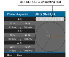
Fig. Phasor diagram window showing the phase sequence according to the direction of the rotary field
