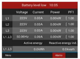
Figures: Device alarm "Battery voltage low"
