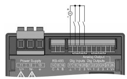
Fig. Connection of digital inputs
