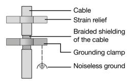
Fig. Shielding design for cabinet entry.
