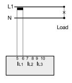
Fig.: Current measurement in a single-phase 2-conductor system
