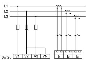
Fig. Connection variant 3w2u - measurement in a threephase 3-conductor network with asymmetrical load.
