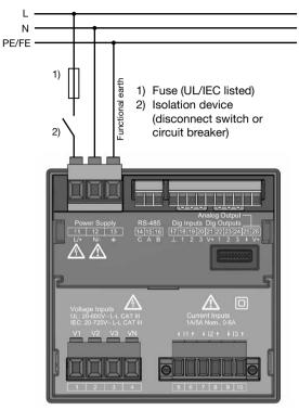
Fig. "Supply voltage" connection example
