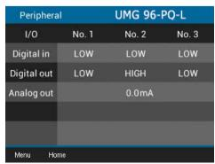
Fig. Displays the states of the digital inputs and outputs and the value of the analog output.
