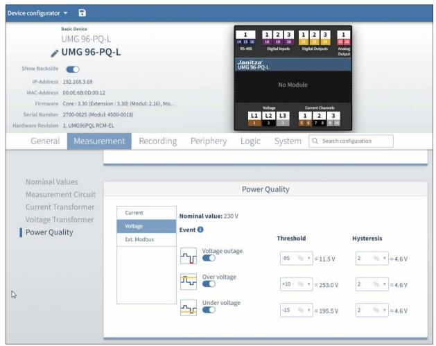
Fig. Configuration of the events in the GridVis software®
