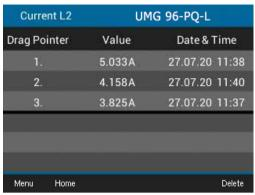
Fig. Drag indicator display - Current L2 (effective) - of the 3 last maximum values with a time stamp.
