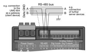
Fig. RS-485 interface, 3-pole plug contact
