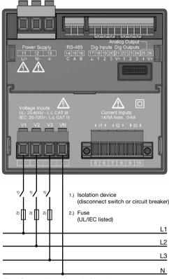
Fig. Connection example for voltage measurement.
