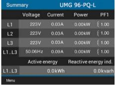
Fig. Measuring display "Summary" - measurement in a three-phase four-wire network (default setting).
