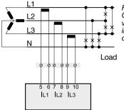
Fig.: Current measurement via current transformer in a three-phase 4-conductor system
