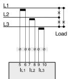
Fig.: Current measurement via current transformer in a three-phase 3-conductor system
