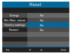
Fig. Reset window, standard factory settings
