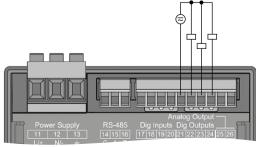
Fig. Connection of digital/pulse outputs
