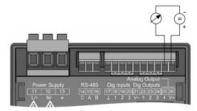
Fig. Analog output connection
