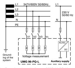
Fig. Example, schematic diagram (UMG 96-PQ-L) -Measurement in three-phase 4-conductor systems.
