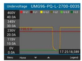
Fig. Sequence visualization of the undervoltage event
