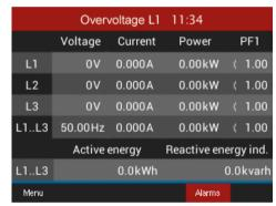
Fig. Example warning message, overvoltage in phase L1.
