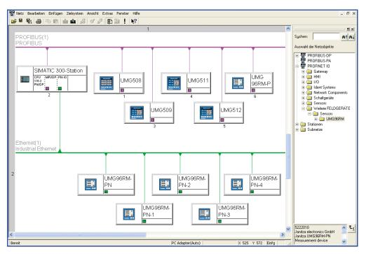
Complete integration of the Janitza measurement devices in the Step  $7^{\circ}$  software environment
