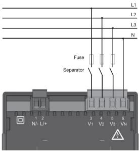
Fig. Connection example for the voltage measurement
