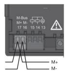
M-Bus interface, 2-pole plug contact
