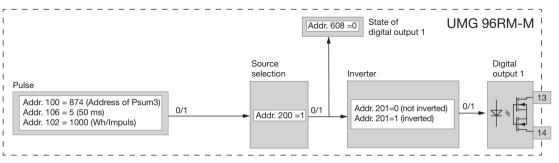
Fig.: Block diagram; Example of digital output 1 as a pulse output.
