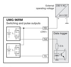
Fig.: Connection example for wiring the pulse output.
