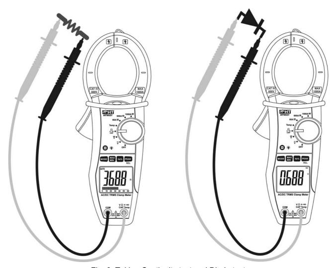
Fig. 6: Taking Continuity test and Diode test
