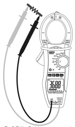
Fig. 5: Taking Resistance measurement
