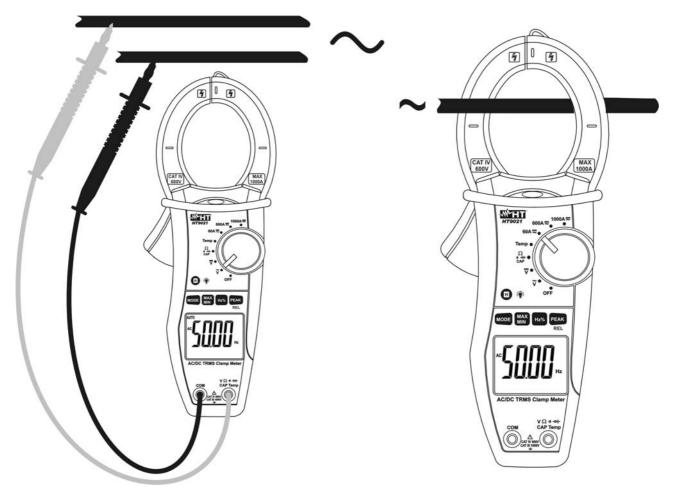
Fig. 10: Taking frequency and duty cycle measurements
