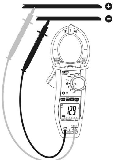
Fig. 4: Taking DC voltage measurements
