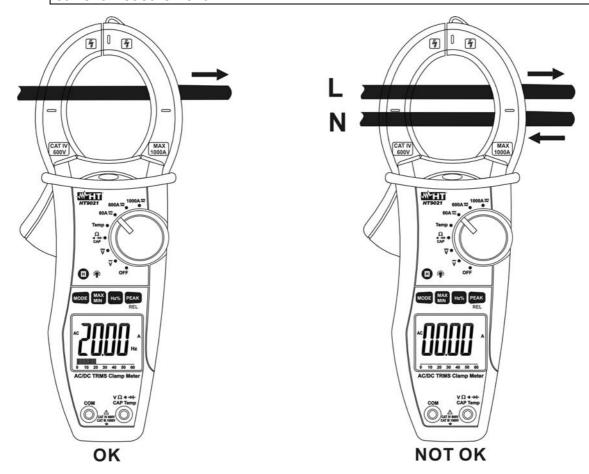
Fig. 9: Taking AC and DC current measurements
