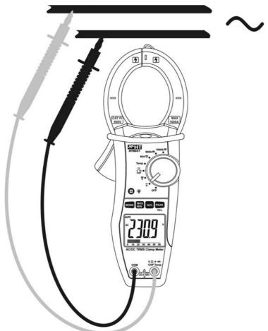
Fig. 3: Taking AC voltage measurements
