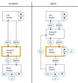
You can toggle between the different displays by using the four device buttons. Depending on the type of display (standard display, alarm display, menu display, info display), the meaning of the buttons is different. The picture below illustrates which button is to be pressed for accessing the individual display. First, you have to distinguish between an alarm condition and no alarm condition.
