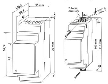
Mount the device vertically, to allow sufficient air flow through the ventilation slots at top and bottom!
