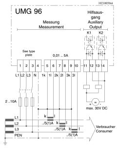
Diagr: Connection example, four wire measurement with three current transformers
